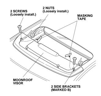
14. Position the moonroof visor with equal spacing on all sides. Check that the rubber seal is not twisted or rolled under the visor.
